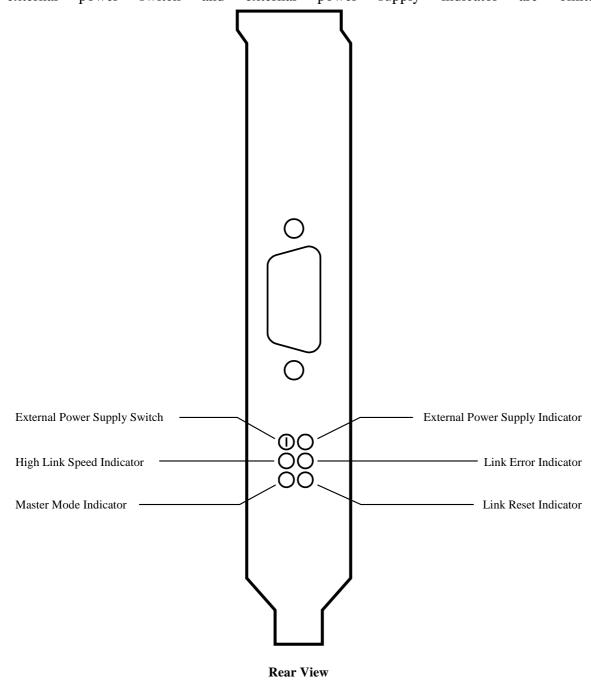
The *external power supply switch* is used to turn the 5V supply on Hema and MSC link connectors on and off by means of a small screwdriver. The red *power supply indicator* lights when power is turned on.
