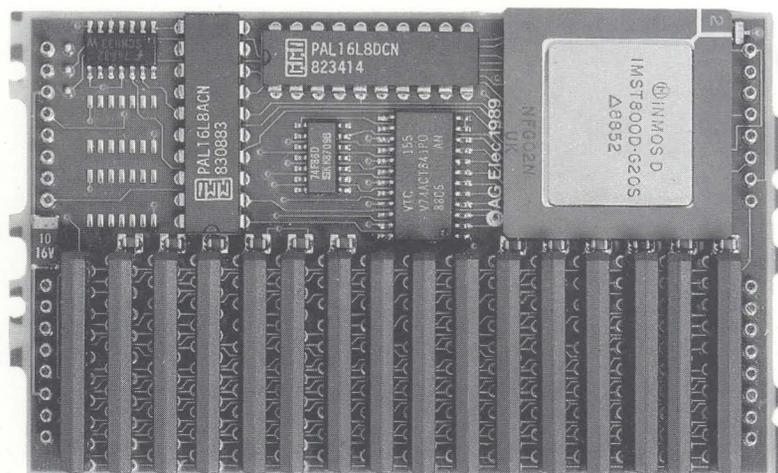
**Introduction** The Transtech TTM6 TRAM (TRANSputer Module) is a small industry standard daughterboard for the Transtech range of TRAM motherboards. It has 2 MBytes of dynamic RAM and is capable of supporting the IMST800, IMST425 and IMST414 transputers. It also has the ability to control a sub-system of transputers.
