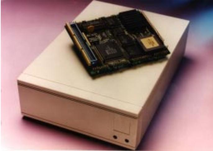
The Matchbox is a small self contained unit allowing up to 4 separate transputer systems to be connected to a UNIX workstation via a SCSI port.
