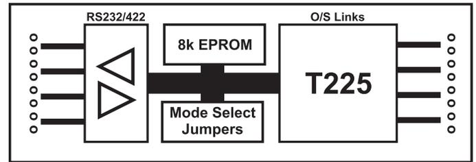
The Transtech TTM21 and TTM23 respectively enable up to four RS232 or RS422 connections per TRAM to be made to a transputer network. The RS232 and RS422 interfaces support serial transfer rates of 9.6Kbaud and can buffer up to 256 bytes internally. This is more than adequate for interfacing a mouse, keyboard, printer or instrumentation.
