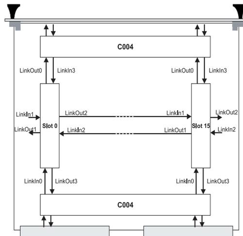
The TMB12 is a double extended Eurocard with slots for up to 16 TRAM modules. The 2 on board IMSC004 link crossbar switches allow the topology of the transputer network to be controlled from software, connecting together the links from the TRAM slots and 32 links which are taken to the edge connectors.
