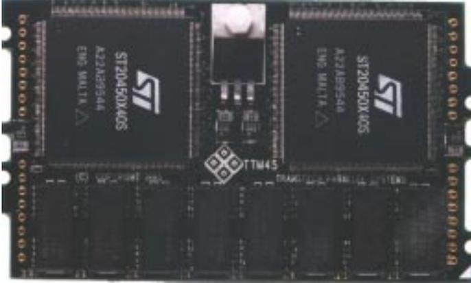
The TTM45 is a size 2 TRAM with two ST20450 processors each with 4Mbytes of fast page mode DRAM. Electrically the TTM45 is two independent size 1 TRAMs, i.e. there are no link connections on the module between the two processors.
